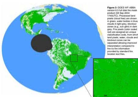
Figure 3. GOES WF\_ABBA version 6.5 full disk fire mask product (08 Sep 2004 1745UTC). Processed land pixels (cloud free) are shown in green, water bodies in blue, clouds in light grey, blackout zones in dark grey, and fire pixels (color coded red) are assigned an unique classification code, from which land pixels, water, clouds and blackout zones can be separated allowing improved interpretation compared to fire-no fire information provided by standard fire location text files.
